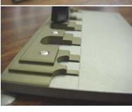
where practice definitely makes perfect! In any case, once the starting point for the bend is determined, the piece is laid on the foam sheet, and a drill bit of the correct diameter is positioned at that location. The bit should have a slightly smaller radius
