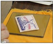
The egg carton foam pad works well for bends of less than 90°. Place the part on the foam sheet, and mark the correct location. Position your blade over the mark and press straight down on the P/E part until it bends to the desired angle. Sounds too simple, doesn't it?
