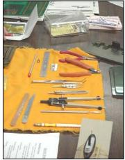
cutting parts off the fret, sheets of foam cut from egg cartons, and an Etch Mate Photo Etch Bending Tool.
